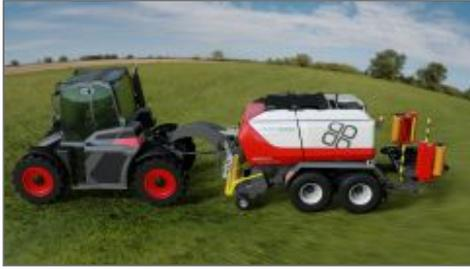
Described by some as a modern take on the Fendt Xylon, and by others as a telehandler without the telescopic arm, all we know is that Austrian firm Syn Trac claims to have developed the ultimate systems tractor. Unveiled in prototype form at Agritechnica, the Syn Trac's main claim to fame is a fully-automatic docking process for front and rear-mounted kit (includes the pto shaft (1000rpm standard), hydraulics, pneumatics, electrics, etc).
