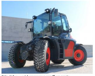
(http://s3-eu-west-1.amazonaws.com/ff-wp-assetslive/sites/1/2017/12/Syn-Trac-01b.jpg) Syn Trac is intended as a high-specification multi-purpose vehicle – the prototype has a 420hp engine and CVT transmission mounted centrally.
