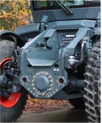
(http://s3-eu-west-1.amazonaws.com/ff-wp-assets-live/sites/1/2017/12/Syn-Trac-02.jpg) A unique couplings interface is used to attach a 3-point linkage or loader module, a trailer or tanker gooseneck drawbar, and a third axle.
