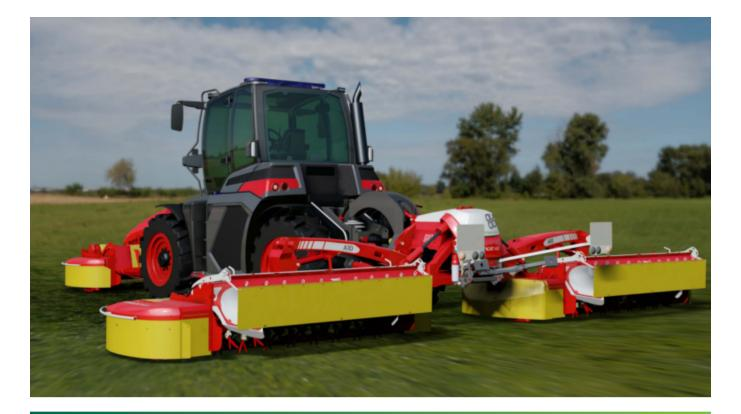
The Syn-Trac runs in permanent 4WD. The standard vehicle is a 4X4 machine; it can be configured as a 6X6 driveline (when an additional axle is 'docked').
