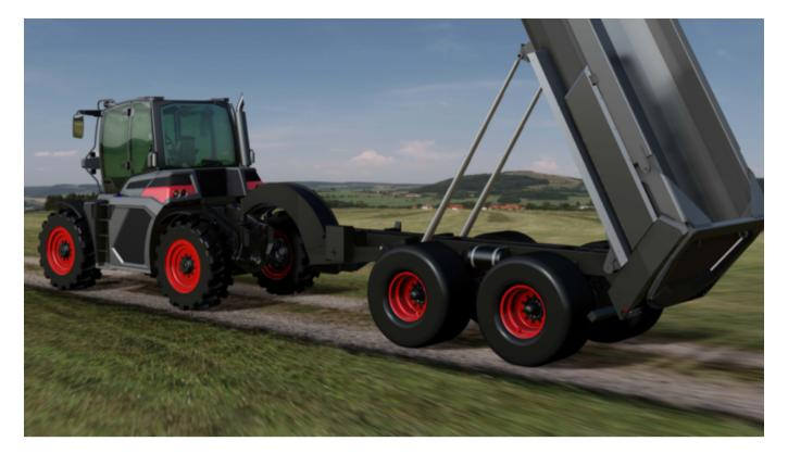
The hydraulic system is fed by a load-sensing, axial-piston pump; maximum output is 180L/min (at 210 bar). The vehicle is home to six double-acting valves; the hydraulic tank can hold 120L.
