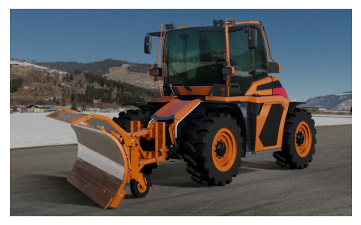
The axles are from Tatra; they incorporate independent suspension – an active, hydro-pneumatic system. Maximum axle loading – for each of the two axles – is a hefty 10t.
