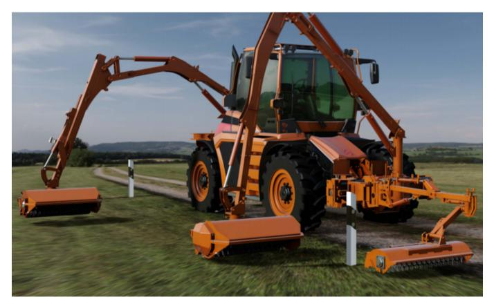
1,000rpm PTOs are standard. There's also a 24V/125A electrical (output) connector. The machine is 2.55m wide; it stands 3.4m high. Depending on tyres, it spans 4.7m in length.
