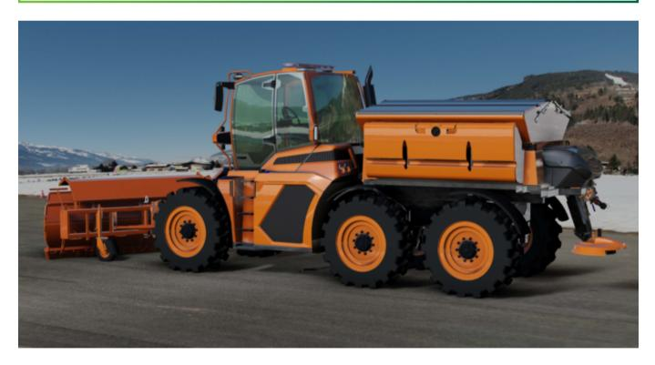
In 4X4 guise, there are multiple **steering modes**, including: front-wheels only; fourwheel steering; and crab steering.
