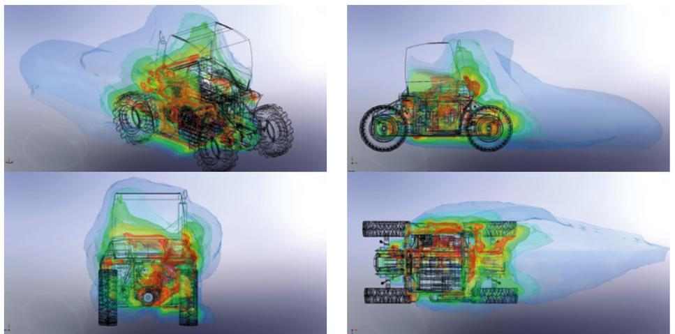
Figure 6 a - d. Analysis of the temperature distribution
