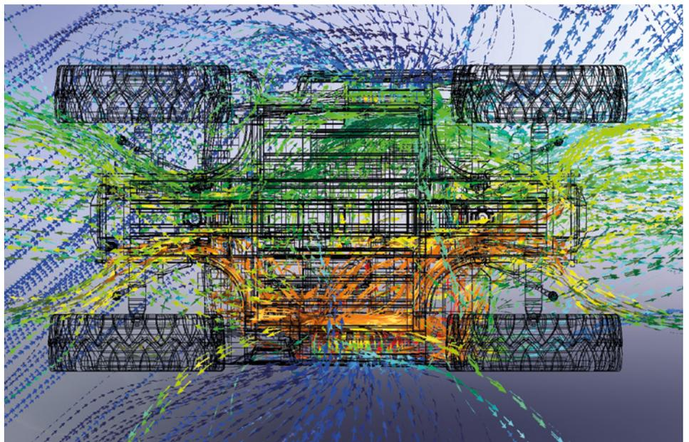
Figure 4. Cooling airflows into the undercarriage
