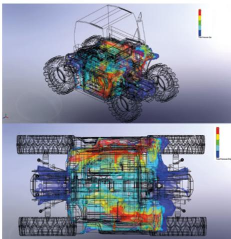
Figure 5 a, b. Analysis of the overpressure areas
