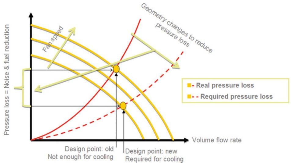
Figure 1. Cooling air vs. pressure loss
