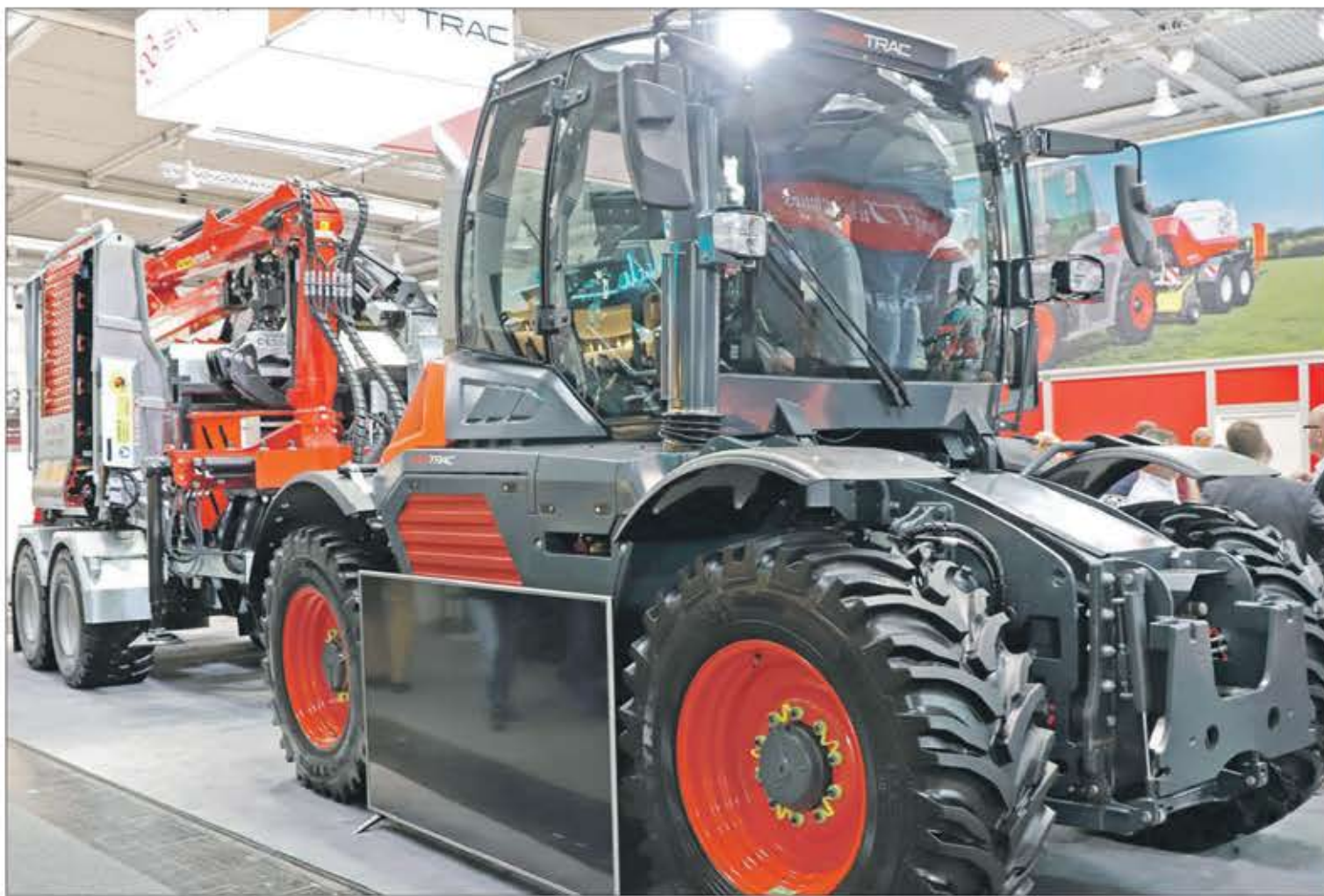
With a 420-horsepower Caterpillar engine, the Syn Trac is capable of handling heavy work loads. During Agritechnica last November it was displayed with a wood chipper. | ROBIN BOOKER PHOTOS
