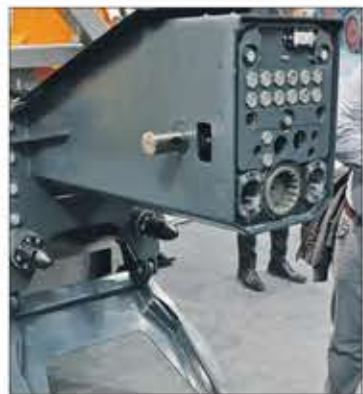
The docking adapter is installed on attachments so that operators can automatically hook up to it without getting out of the cab. Hydraulic lines, the power take-off and electrical components all connect by the push of a button.
