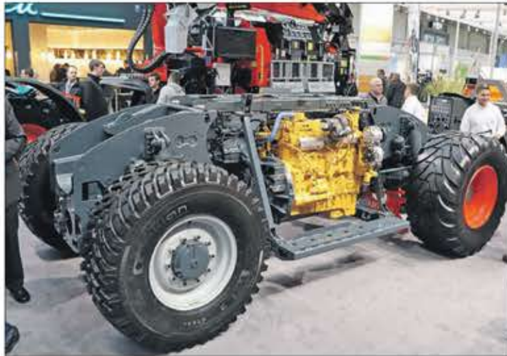
The engine and hydro-mechanical power split transmission are located in the centre of the machine, underneath the cab.
