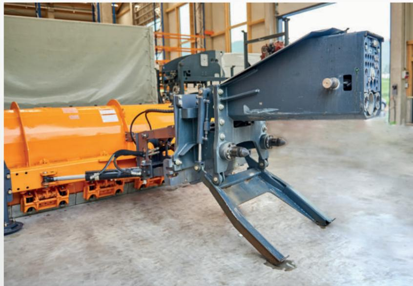
Seven interfaces are connected automatically in under a minute – with just one person who doesn't have to leave the driver's cabin.
