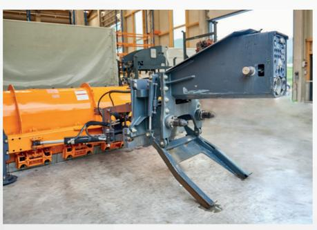
Seven interfaces are connected automatically in under a minute – with just one person who doesn't have to leave the driver's cabin.
