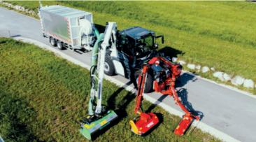
One SYN TRAC rig instead of three special purpose vehicles: the comfortable oneman operation of both attachments facilitates vertical and horizontal hedge trimming, including vacuuming of cuttings.
