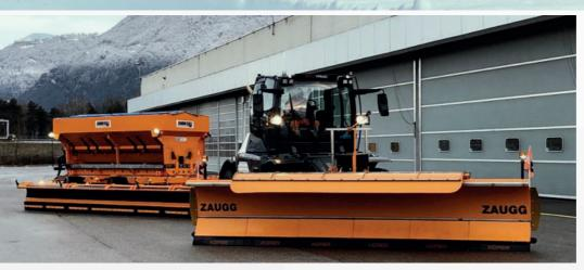
Visibility and mobility also pay off in winter services. Thanks to hydrostatic-mechanical transmission, the scope of performance for gritting applications is equivalent to that of a self-propelled snowblower.
