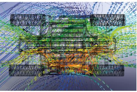
Figure 4. Cooling airflows into the undercarriage
