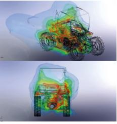
Figure 6 a - d. Analysis of the temperature distribution
