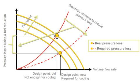
Figure 1. Cooling air vs. pressure loss
